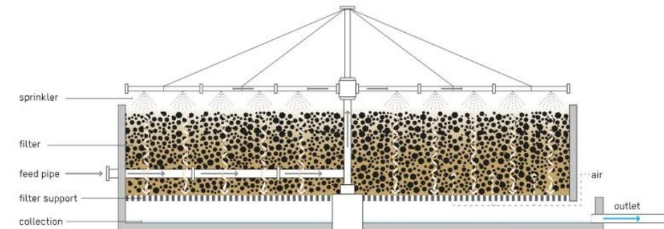
Figure 23: Trickling Filter system (Tilley, 2014)
