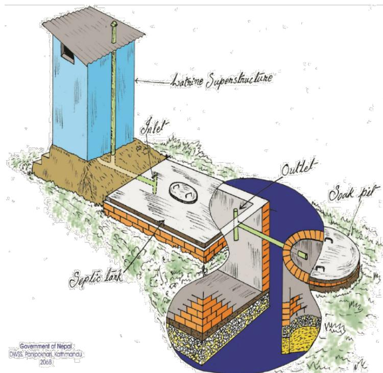
Figure 10: Scientific Septic Tank with Soak Pit (DWSS)
