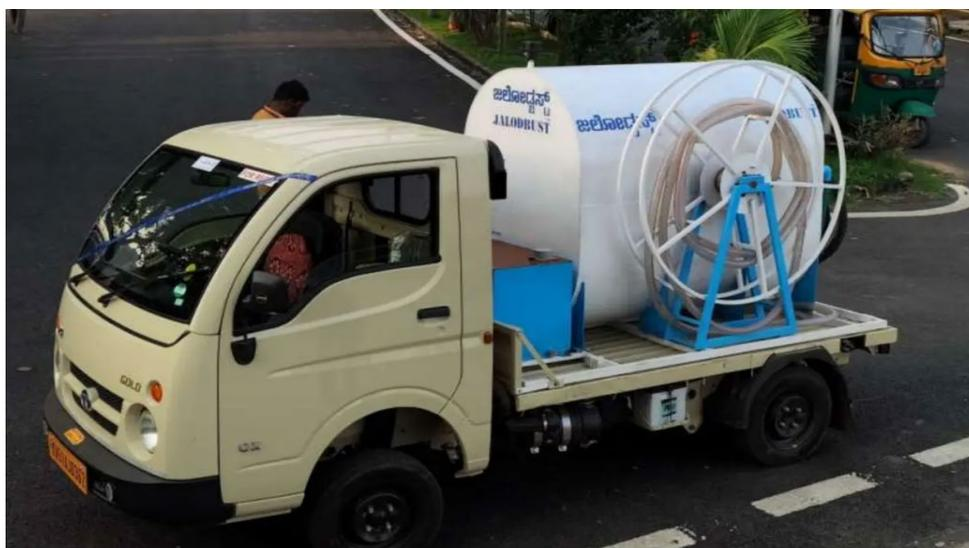
Figure 13: Vehicle mounted compact emptying system: (JALDOBUST(R), 2024)
