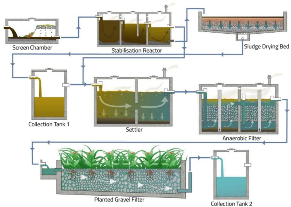
Figure 20: Reconfigured DEWATS for FS treatment
