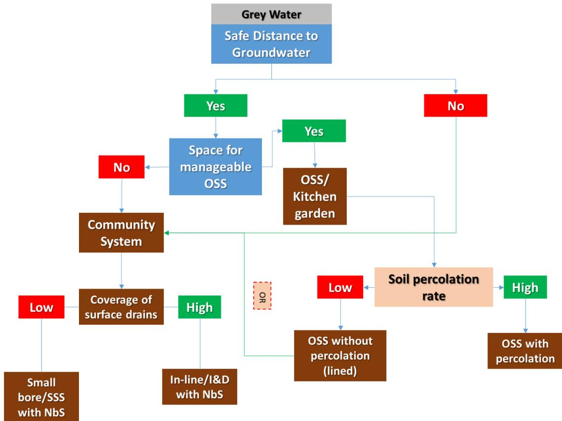
Figure 9: Methodology for choosing the suitable technology options for greywater management
