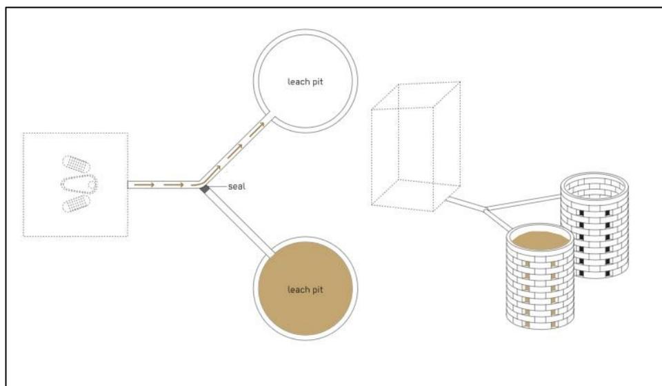
Figure 11: Twin Pit System for Pour flush toilets (Tilley, 2014)
