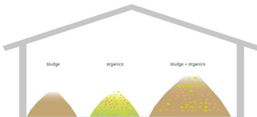
Figure 30: Co-composting with wet solid waste (Tilley, 2014)
