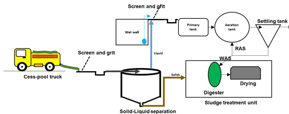
Figure 28: Solid-liquid separation method
