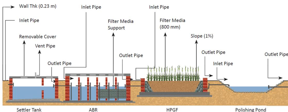
Figure 19: Decentralized Wastewater Treatment Systems (DEWATS)
