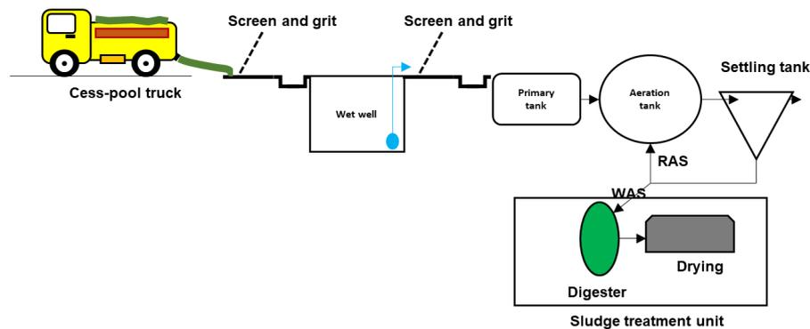
Figure 27: Direct addition method
