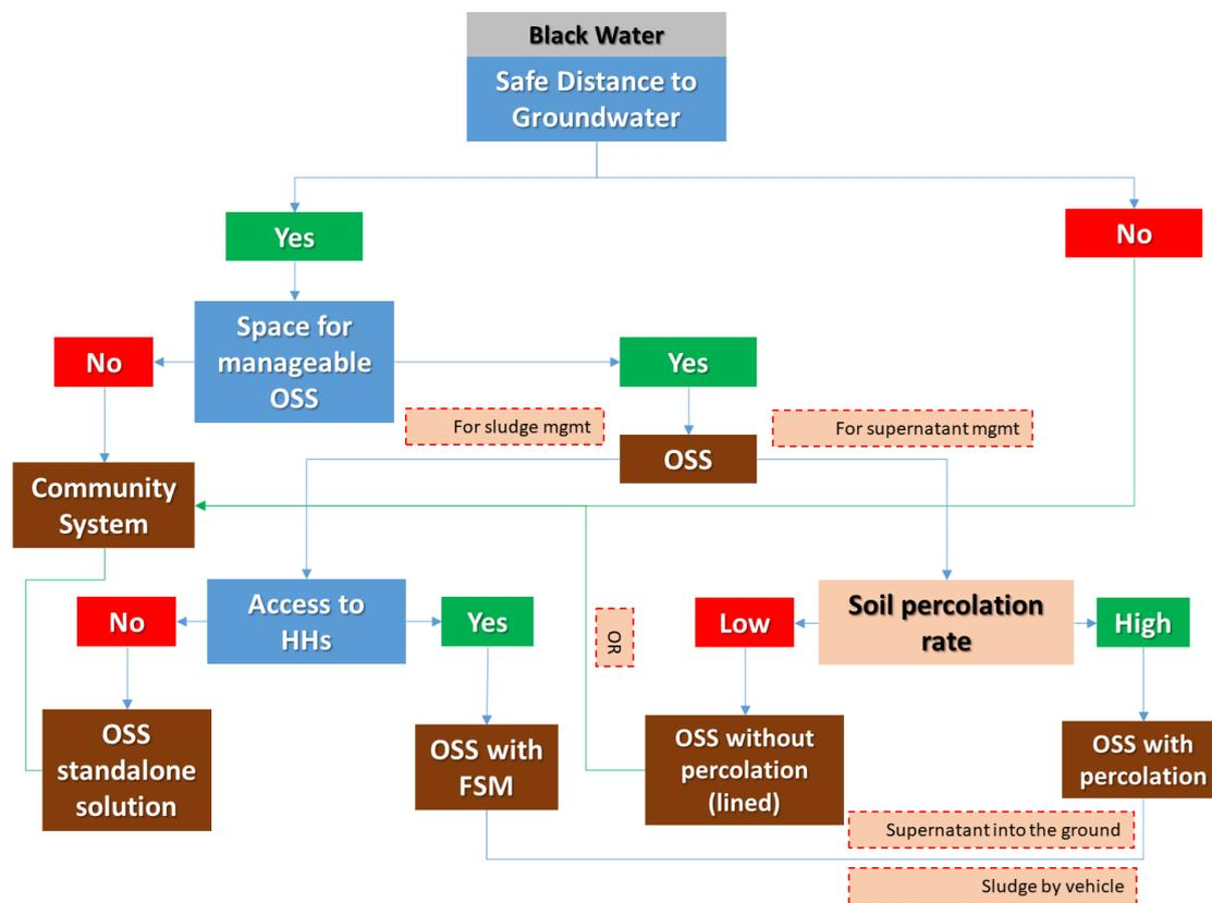
Figure 8: Methodology for choosing the suitable technology options for blackwater management
