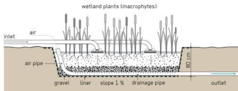
Figure 22: Constructed Wetland System (Tilley, 2014)
