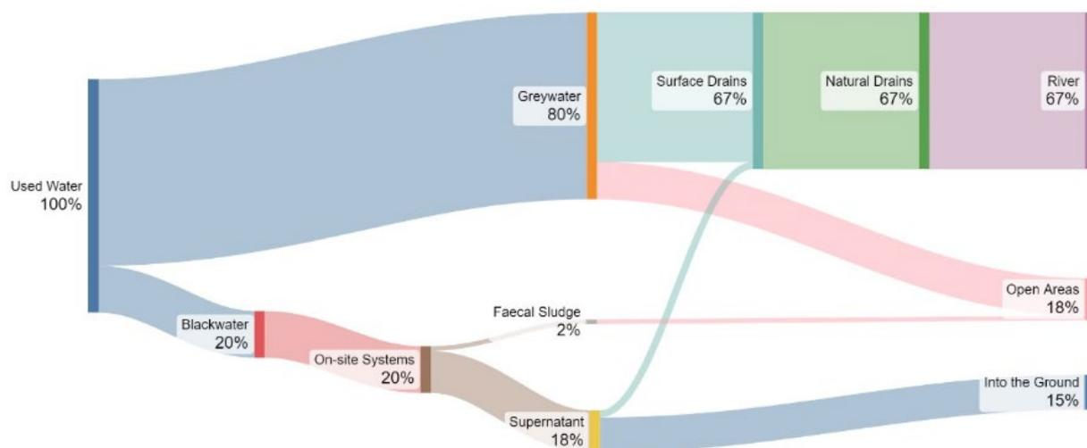
Figure 5: San-key Diagram illustrating usedwater flows across the service chain for the town of Barkot
