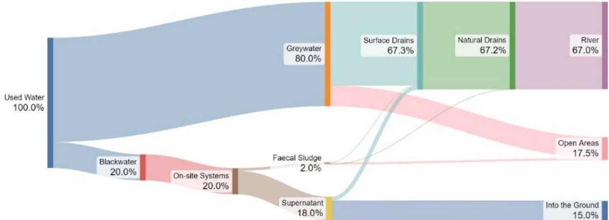
Figure 3: San-key Diagram illustrating usedwater flows across the service chain for the town of Champawat
