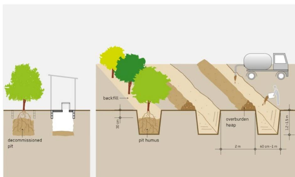
Figure 31: Trenching (shallow and deep row) for safe disposal of fecal sludge (Tilley, 2014)
