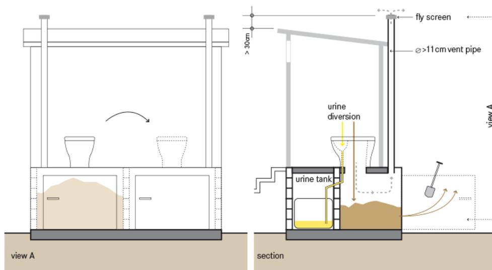
Figure 12: EcoSan Toilets with urine diversion (Wateless) (Tilley, 2014)
