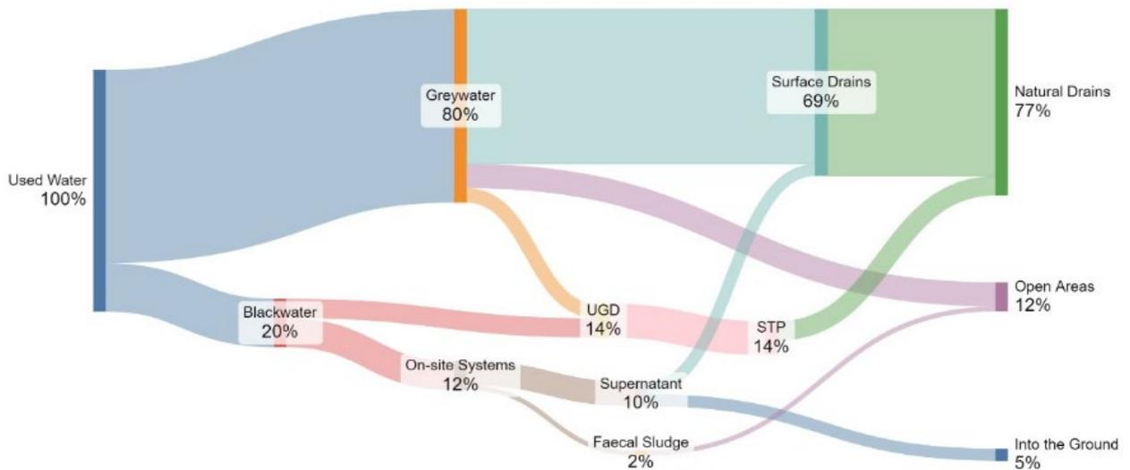
Figure 4: San-key Diagram illustrating usedwater flows across the service chain for the town of Mussoorie
