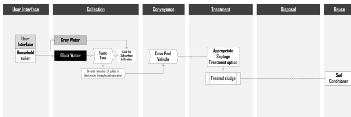
Figure 2: The flow chart illustrating the usedwater management in non-networked systems
