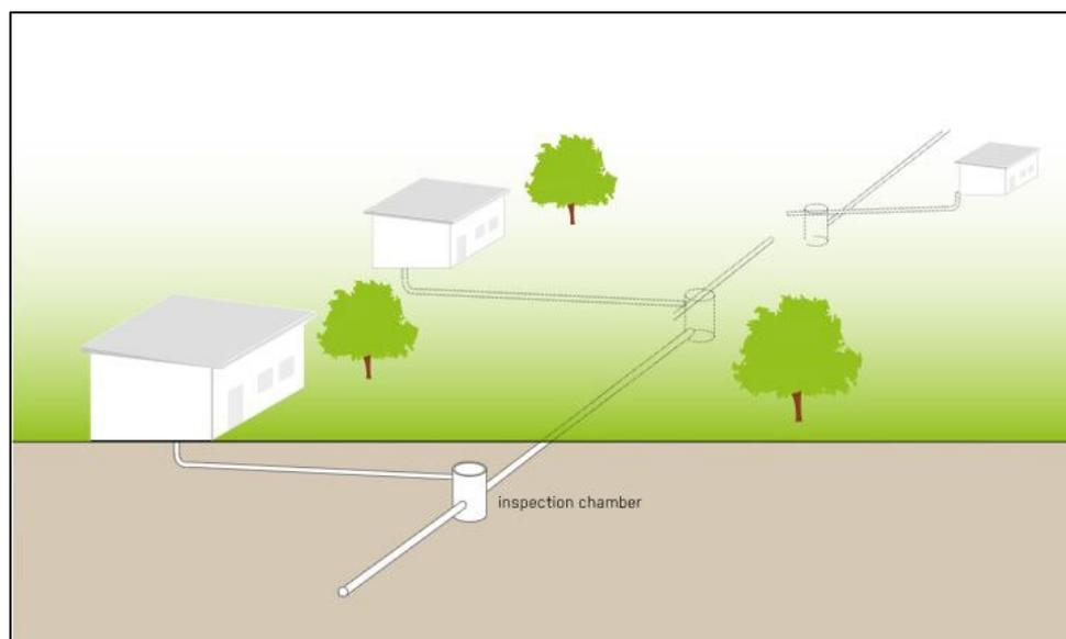
Figure 14: Simplified sewer system (Tilley, 2014)
