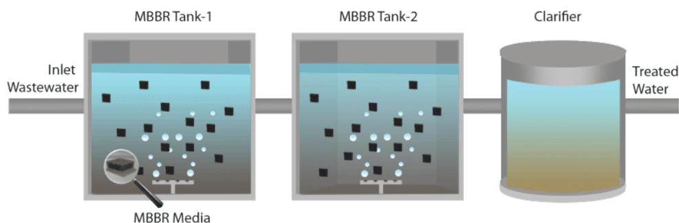
Figure 24: Moving Bed Biofilm Reactor (MBBR)
