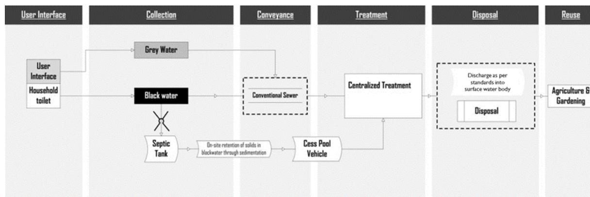
Figure 1: The flow chart illustrating the usedwater management in networked systems
